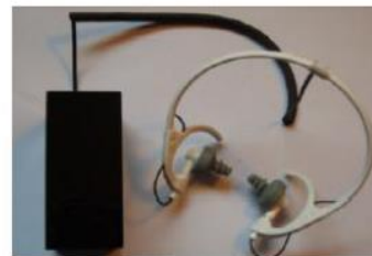
Headphone Developed Solid Model - Aquaeye™ Designed and Developed Swimmers Radio Headset
