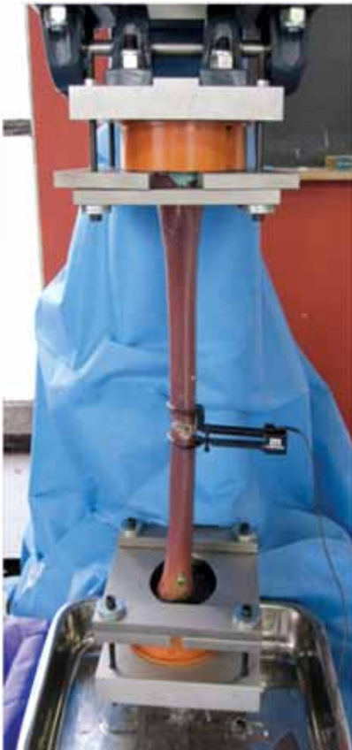
A synthetic shin bone with an IM nail inserted is shown mounted on one of CIT's mechanical testing machines. A measurement device called an extensometer was attached around the fracture to record the motion between the bone fragments while the machine applied loads representative of walking. Similar tests were performed on prototypes of the novel IM nail
