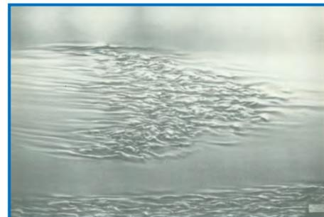
Figure 4.15 Turbulent Spots (NTU, 2011)
