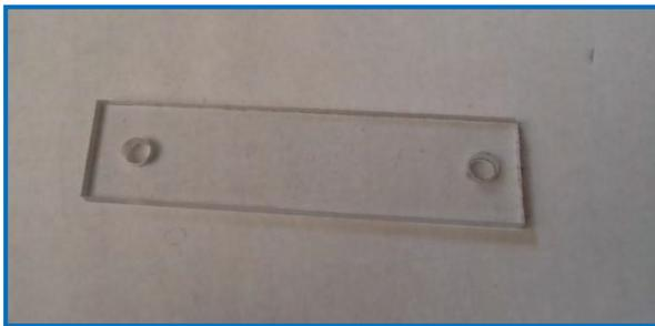
Figure 7.51 Calibration test piece (Hand, 2014)
