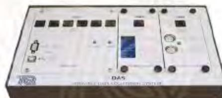
Versatile Data Acquisition System Bench-top Interface (VDAS-B)
