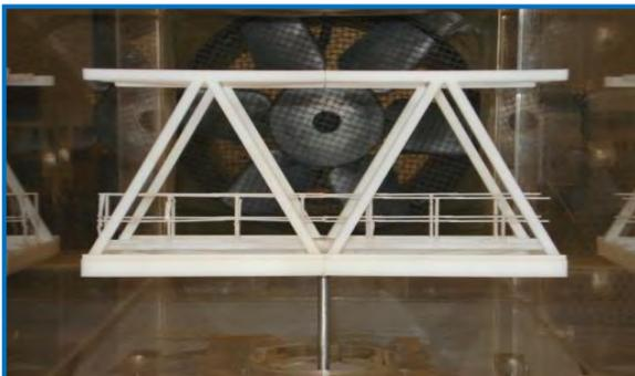
Figure 6.41 Model aligned with airflow
