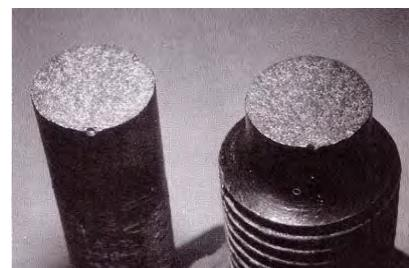
Figure 3.7 Brittle-failure
