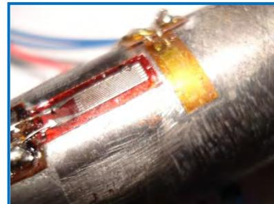
Figure 7.105 Strain gauges on shaft (*Hand, 2014*)
