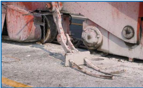
Figure 7.1 Failure of tie-down system (Liftech, 2009)
