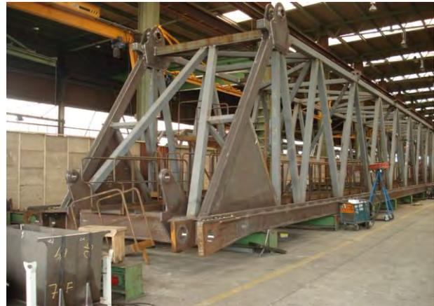
Figure A-2 Hinge point mechanism on boom
