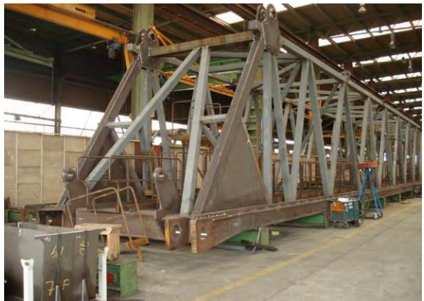
Figure A-2 Hinge point mechanism on boom section
