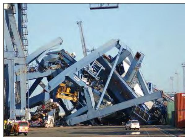
Figure 3.3 Toppled crane after storm (*Vertikal, 2008*)
