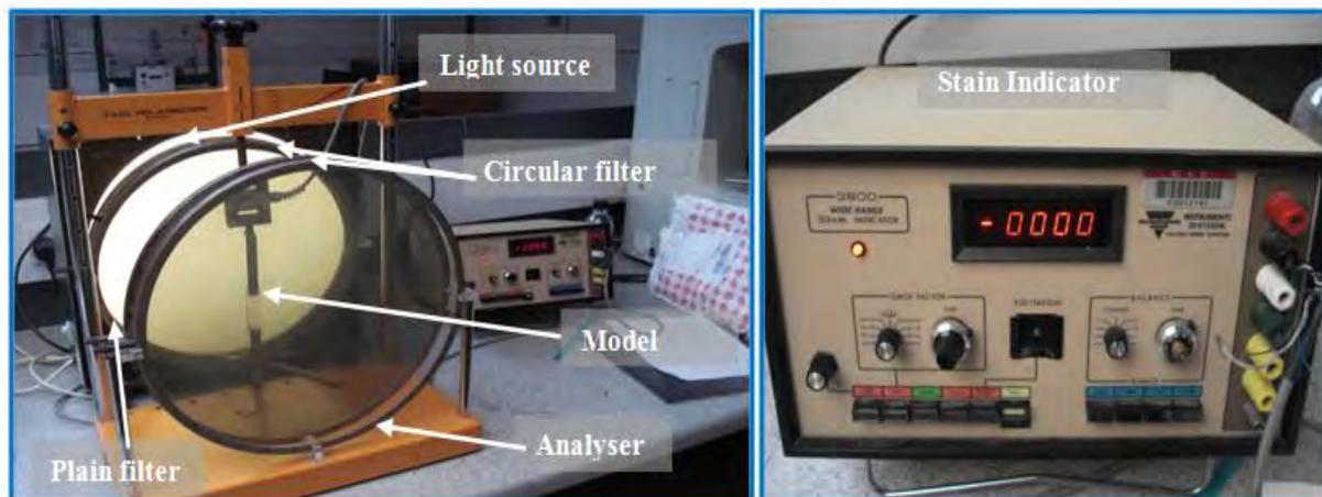
Figure 7.49 College circular polariscopes equipment (Hand, 2014)
