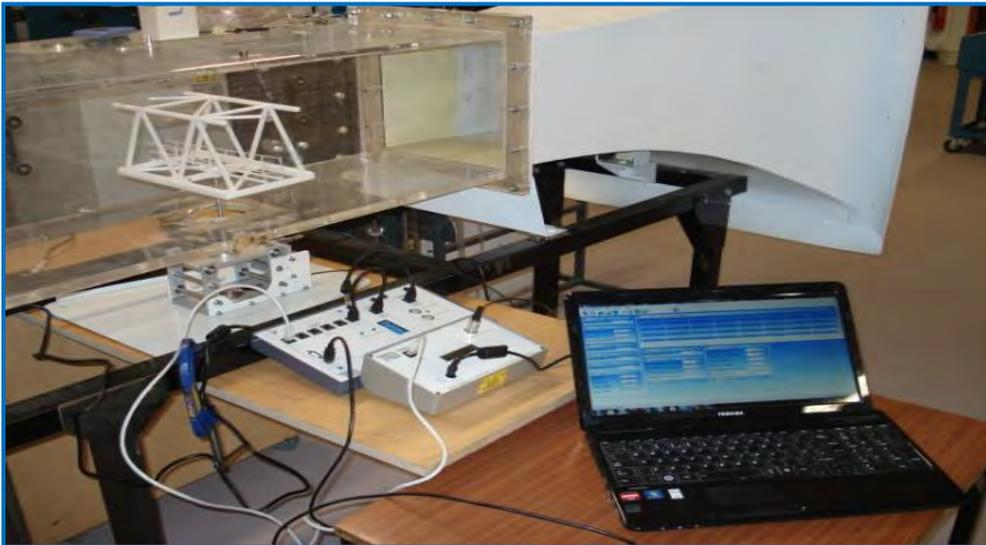
Figure 6.43 VDAS enabled with force balance and controlled with a laptop
