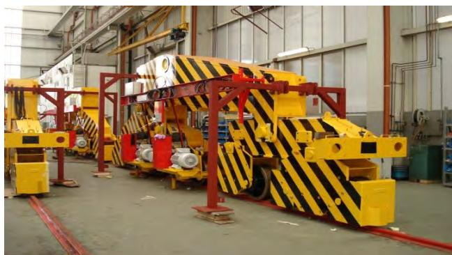
Figure A-8 Crane's Travel Unit (*Hand, 2013*)
