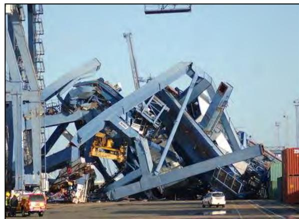
Figure 3.3 Toppled crane after storm (Vertikal,2008)
