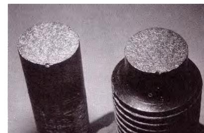
Figure 3.7 Brittle-failure (Warnes, 2006)
