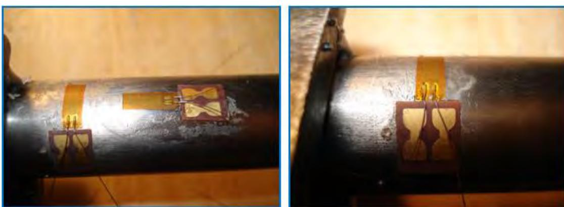
Figure 7.85 Strain gauge orientation (L) & Lateral orientated strain gauge (R) (Hand, 2014)
