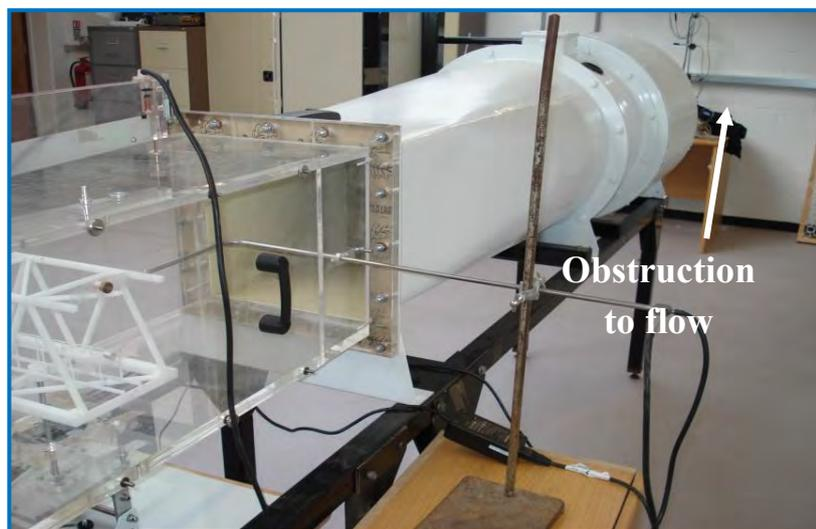
Figure 6.59 Wind Tunnel exit (*Hand, 2014*)
