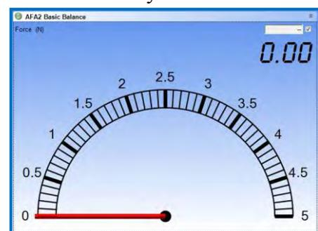
The data acquisition system software allowed the monitoring of drag values using a digital dial during the wind tunnel testing and could be data logged to allow post-processing of the results at a later date.
