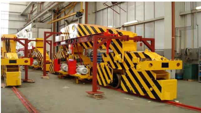
Figure A-8 Crane's Travel Unit (Hand,2013)
