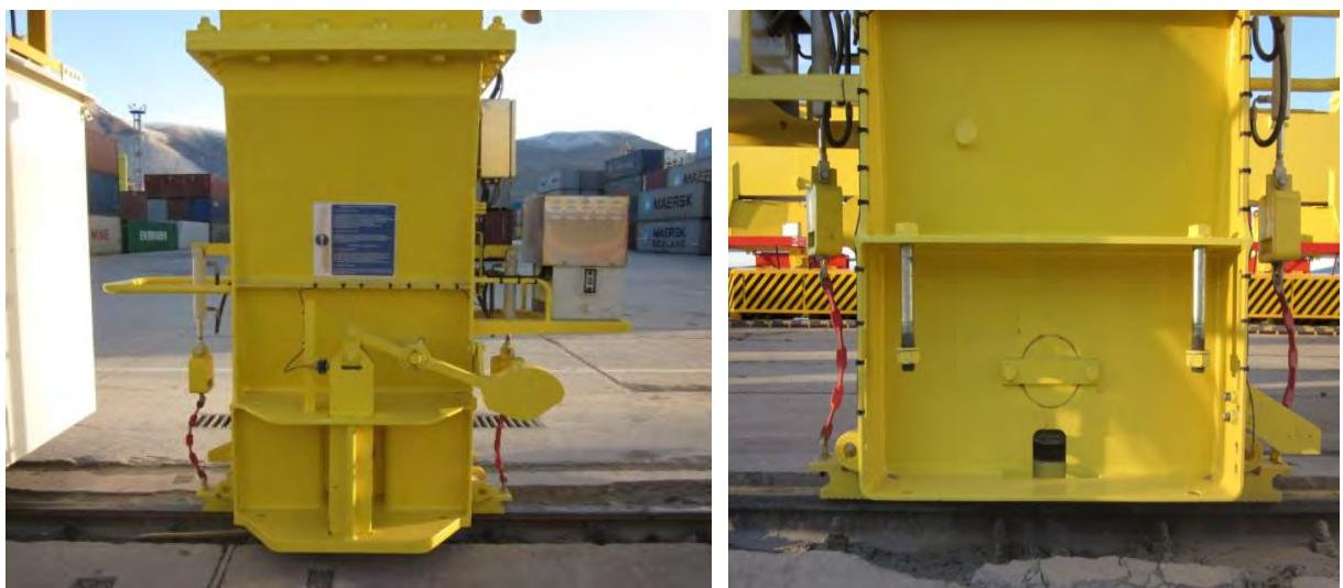
Figure A-10 Crane storm anchor from under sill beam (*Liebherr Group, a 2013*)
