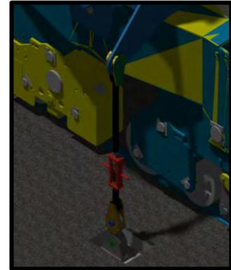
Figure 7.0 Current Tie down system (Hand, 2013)
