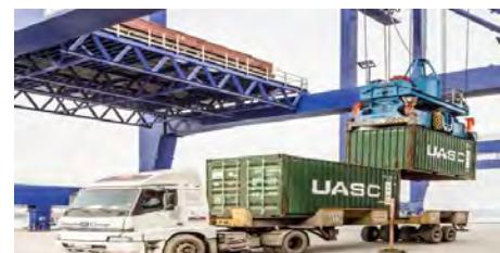
Figure 2.3 Container lifted off truck (Liebherr, 2013)
