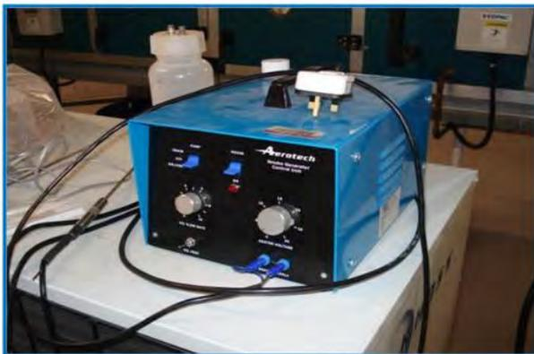
Figure 6.50 Smoke generator used (Hand, 2014)
