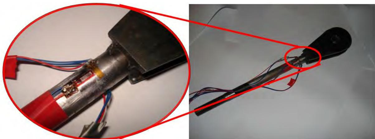
Figure 7.87 Strain gauge position
