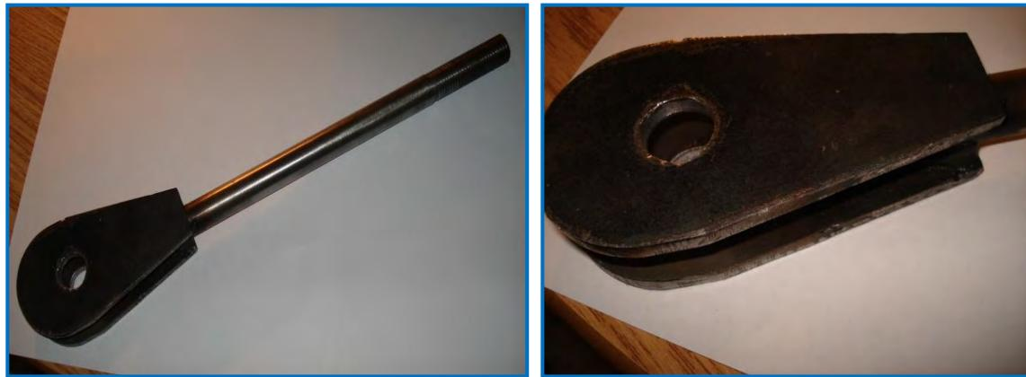
Figure 7.78 Top link and bearing plates (*Hand, 2014*)
