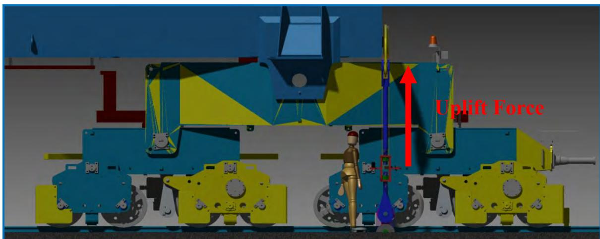
Figure 7.18 Uplift Force at crane corner base unit (*Hand, 2014*)
