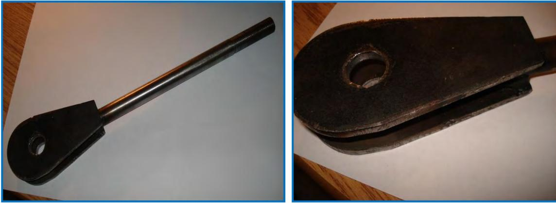
Figure 7.78 Top link and bearing plates (Hand, 2014)
