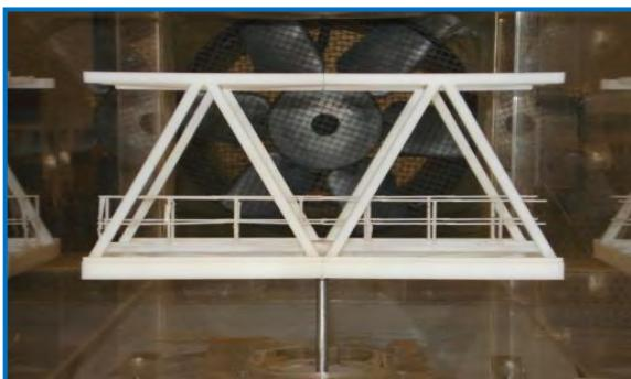
Figure 6.41 Model aligned with airflow
