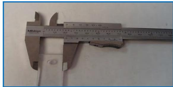
Figure 7.52 Measuring test piece (Hand, 2014)
