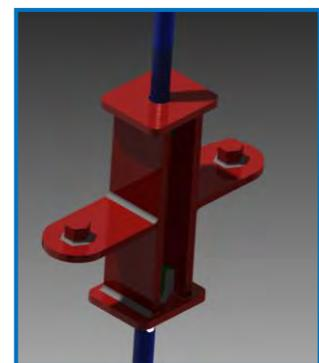
Figure 7.33 Turnbuckle centre (Hand, 2014)
