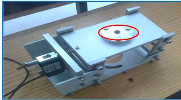
Figure 6.6 Force balance attachment (*Hand, 2013*)
