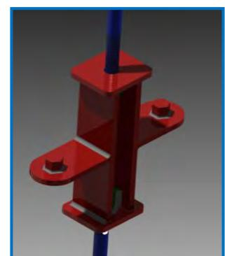
Figure 7.33 Turnbuckle centre (Hand, 2014)
