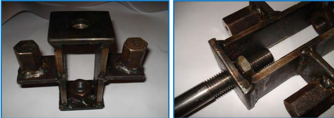
Figure 7.79 Turnbuckle (Hand, 2014)
