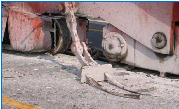
Figure 7.1 Failure of tie-down system
