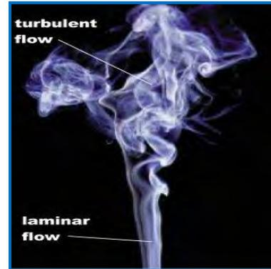
Figure 4.11 Transition of laminar flow to turbulent flow (MIT, 2002)
