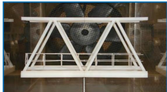
**Figure 6.4 Model showing clearance between wind tunnel walls (*Hand, 2014*)**
