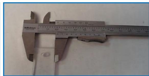
Figure 7.52 Measuring test piece (*Hand, 2014*)
