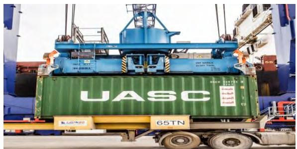
Figure A-6 Head block & spreader connected to a container (Liebherr Group, a 2013)
