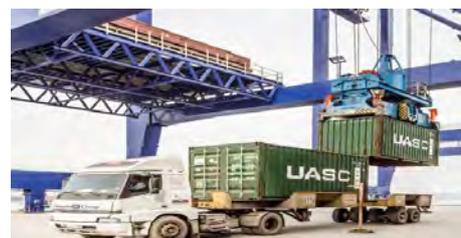
Figure 2.3 Container lifted off truck (Liebherr, 2013)
