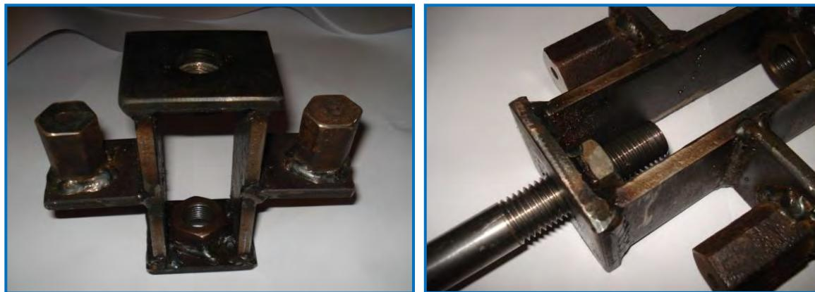
Figure 7.79 Turnbuckle (*Hand, 2014*)
