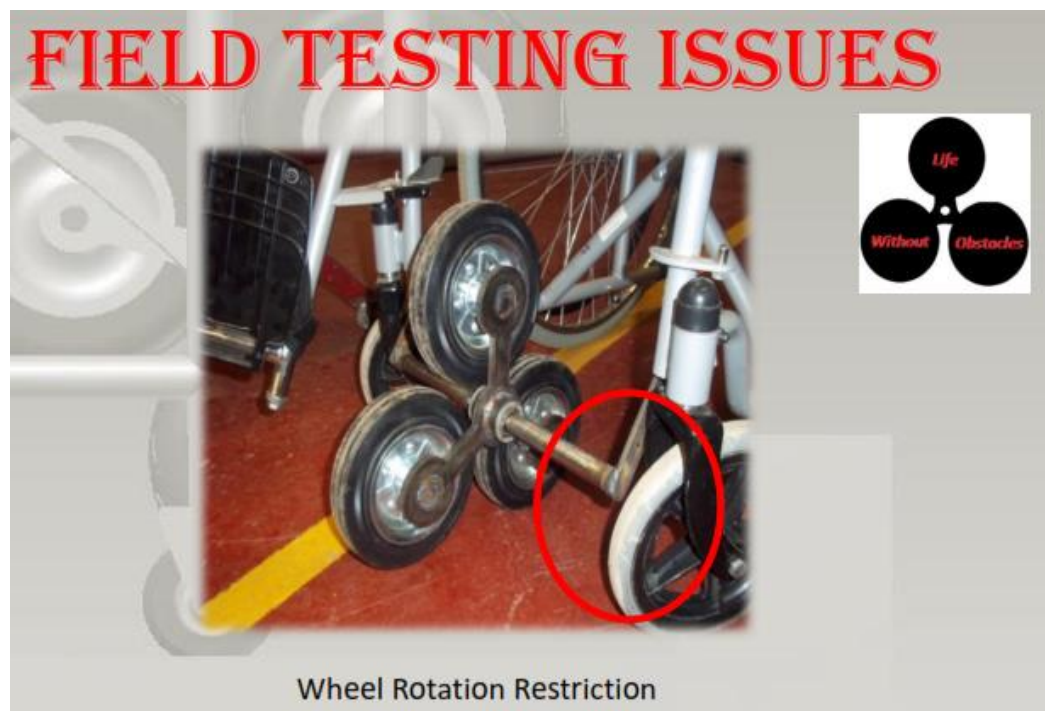
Figure 27 Pyra-Aid™ Mark 1 Prototype Field Testing Castor Wheel Rotation Restriction
