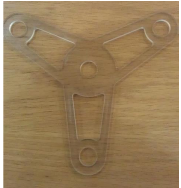
Figure 51 Mark 1 and Mark 2 /3 Photoelastic Structural Models CNC Machined from Sheet PSM-1 Polycarbonate J. Roberts
