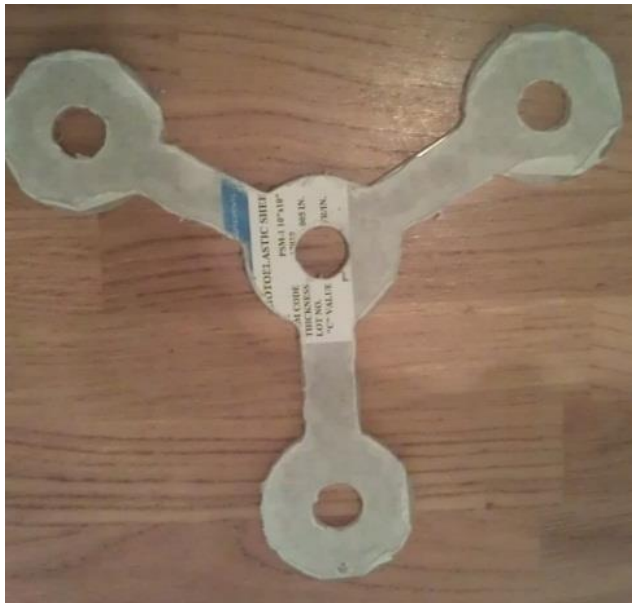
Figure 51 Mark 1 and Mark 2 /3 Photoelastic Structural Models CNC Machined from Sheet PSM-1 Polycarbonate J. Roberts
